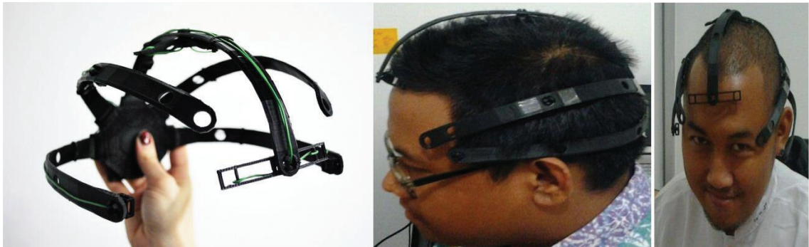
Figure 2. (a) 3d printed OpenBCI headwear. (b) Prototype used by respondent (c) The size is too large for some users
